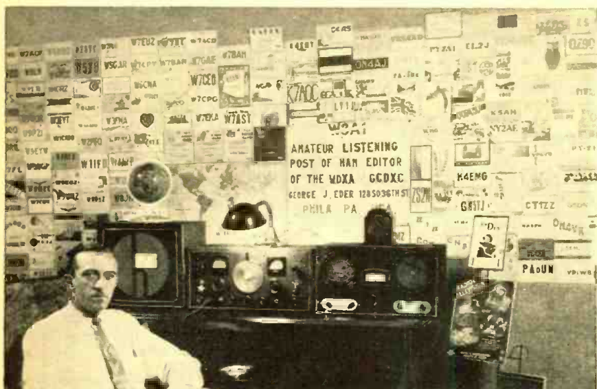
GEORGE J. EDER , 128 So. 36th St., Philadelphia is "HAM" Editor of WDXA and GCDXC, member Radex Club, and of the Short Wave League. His layout comprises a 20 meter ½ wave doublet, an RSR-Clipper Receiver, an SX-16 receiver, and a 12 PM Hallicrafter's Speaker. On phone, he has heard 103 Countries, of which 50 are verified. Forty-five states are also verified on 20 m. fone, out of 48 heard. He has been DXing on the broadcast band since 1920, the Amateur band since 1935, and QSLing Ham stations since 1937. He has 230 cards, and wants to QSL all states of U. S. and all countries heard on 20 meter fone, all states on 10 meter and 75 meter phone.
