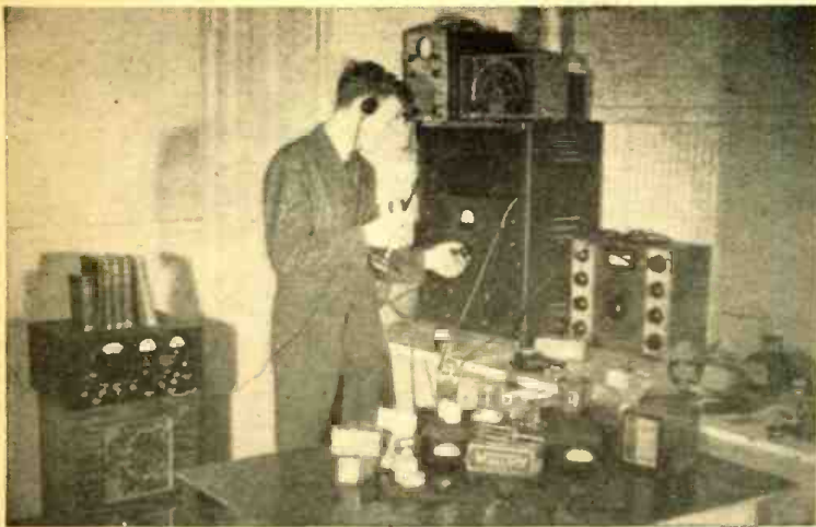
Picture at left shows test laboratory where the R. & T. "pull-swing" F-M system has been developed. Below—close-up of the parts used in building the amplifier here described. A high frequency amplifier, to operate efficiently on 59.2 mc., requires carefully selected parts. The Hallicrafter 527 receiver used in checking the R. & T. "pull-swing" apparatus is shown at the extreme left.
